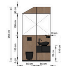
BATHROOM | WALL SECTION 2
